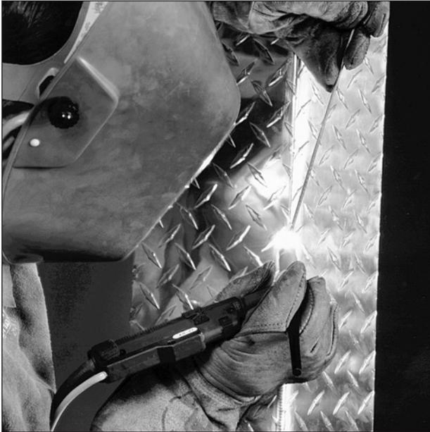
Figure 8.9 Welding in the vertical position.
