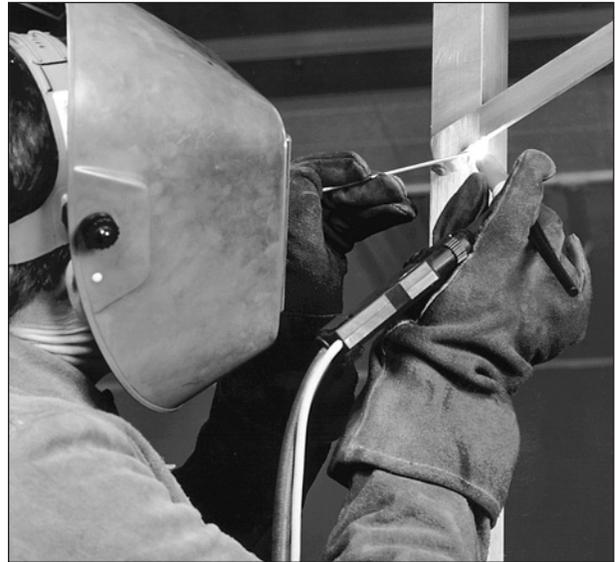
Figure 8.10 Welding in the overhead position.
