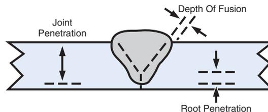
**Figure 7.3** Depth of fusion and types of penetration. Complete joint penetration refers to weld metal that extends completely through the groove and has complete fusion into the base metal. What is shown is a partial joint penetration, which if not intended is referred to as incomplete joint penetration.
