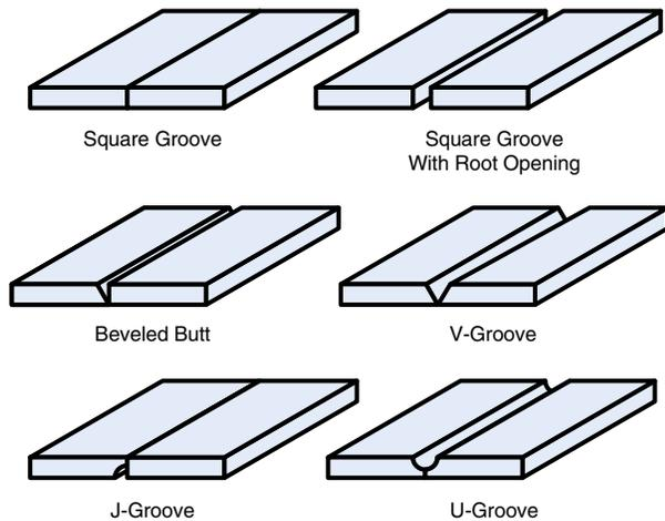
Figure 7.4 Butt joints.
