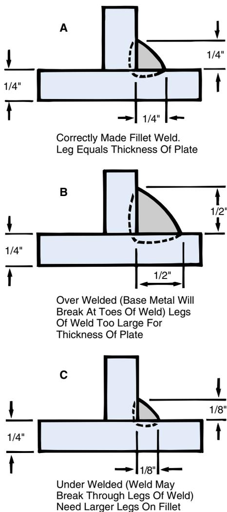
Figure 7.13 Correct/incorrect fillets.
