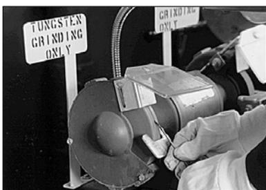
**Figure 4.10** Tungsten electrode preparation.
