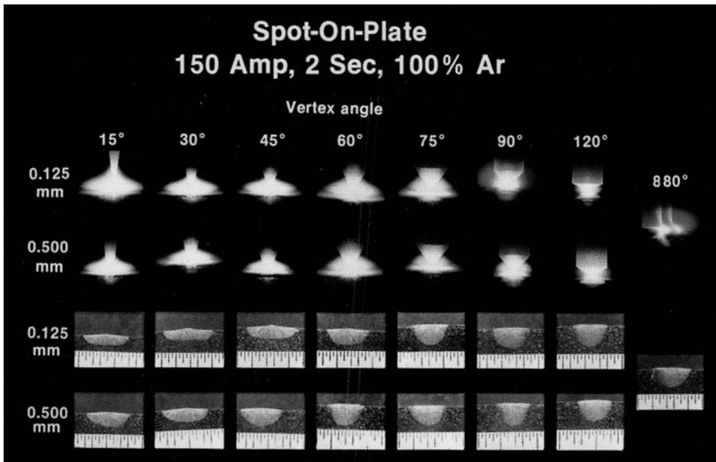
**Figure 4.8** Arc shape and weld profile as a function of electrode tip angle. Image courtesy of *American Welding Society (AWS) Welding Handbook, 8th ed., Volume 2, "Welding Processes."* Miami: American Welding Society.
