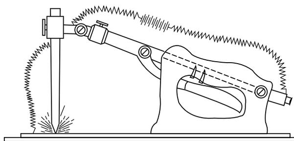
Figure 2.1 Original carbon electrode welding apparatus — 1885.
