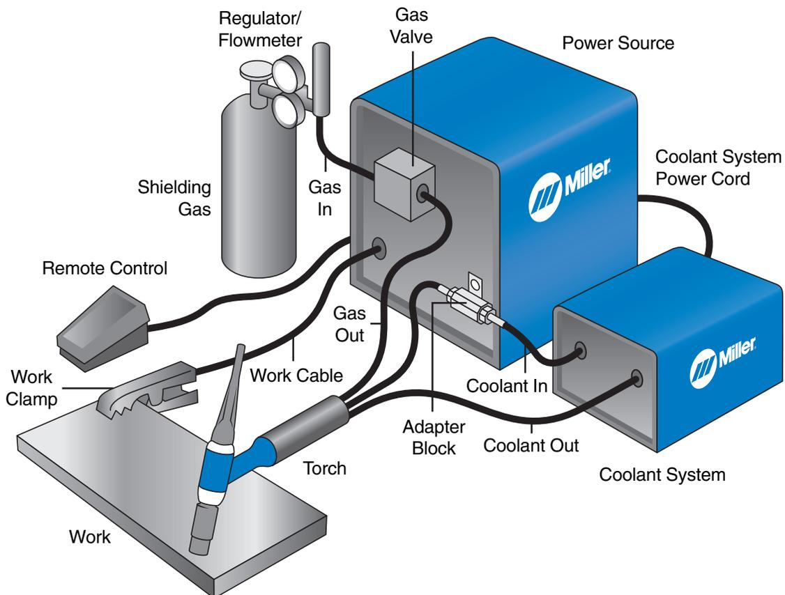
Figure 1.1 Essentials of the GTAW process (water cooled).
